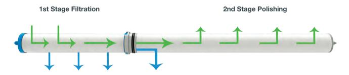
Product enters the filter from an outside to inside flow. The filter then removes solids, semi-solids and large liquid droplets. The second stage of removal is inside to outside flow, aiding in the coalescing of ultra-fine liquids into larger droplets which are then drained into the sump.
